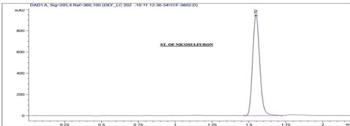
**Figure 5.** HPLC chromatogram of nicosulfuron standard (400 $\mu$ g/mL) at  $\lambda$  = 205 nm.
