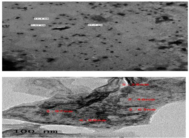
Figure 1. Individual primary ZnO nanoparticles and aggregates were observed under the transmission electron microscope.
